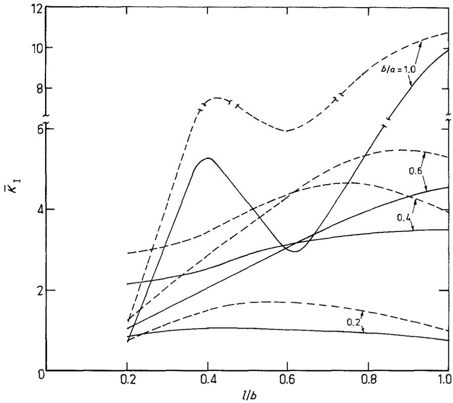
Figure 6 The stress-intensity factor  $\bar{K}_I$  for the applied strain (Equation 62).  $\lambda_1/\lambda = 20$ , and  $\nu = \nu_1 = 0.3$ . (Solid lines represent  $x_2 > 0$  side of debond and broken lines  $x_2 < 0$  side of the debond.)
