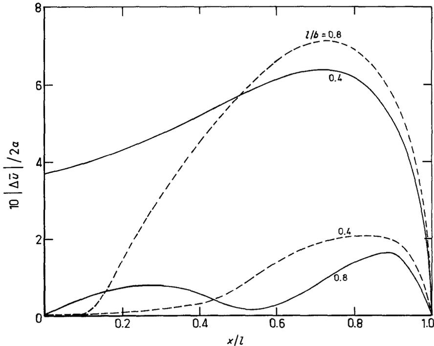
Figure 5 Relative displacements of the debonded faces due to Equation 60.  $\lambda_1/\lambda = 20$ ,  $b/a = 0.8$  and  $\nu = \nu_1 = 0.3$ .
