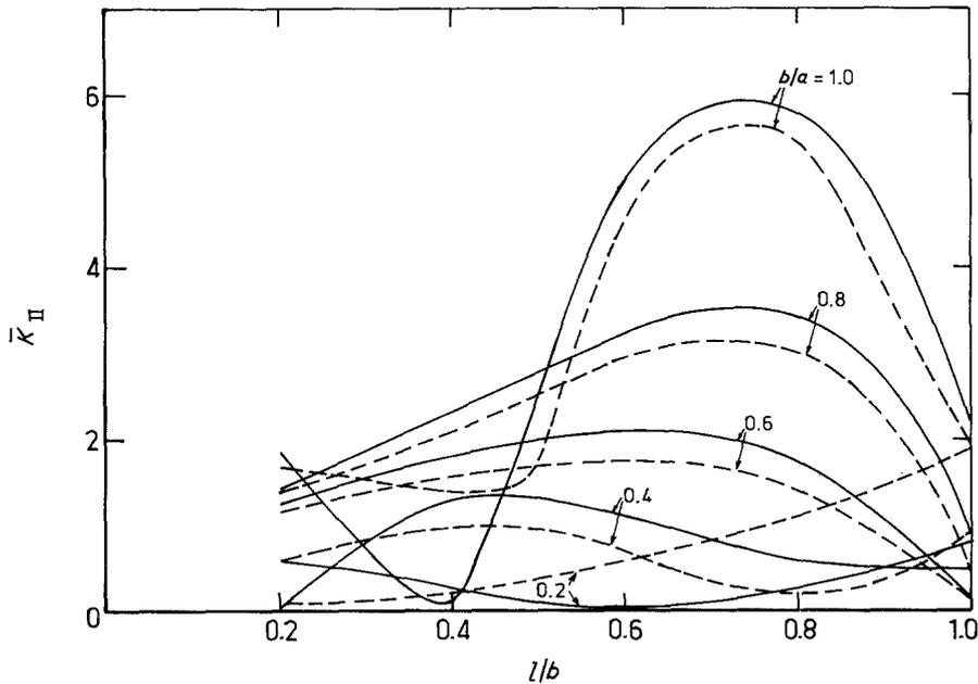
Figure 3 Stress-intensity factor  $\bar{K}_{II}$  arising from Equation 60. Key as in Fig. 2.
