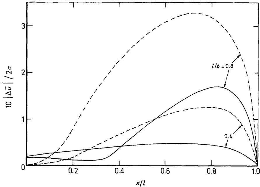
Figure 4 Relative displacements of the debonded faces due to Equation 60.  $\lambda_1/\lambda = 20$ ,  $b/a = 0.4$  and  $\nu = \nu_1 = 0.3$ . Normal displacements are shown by solid lines and tangential displacements by broken lines.
