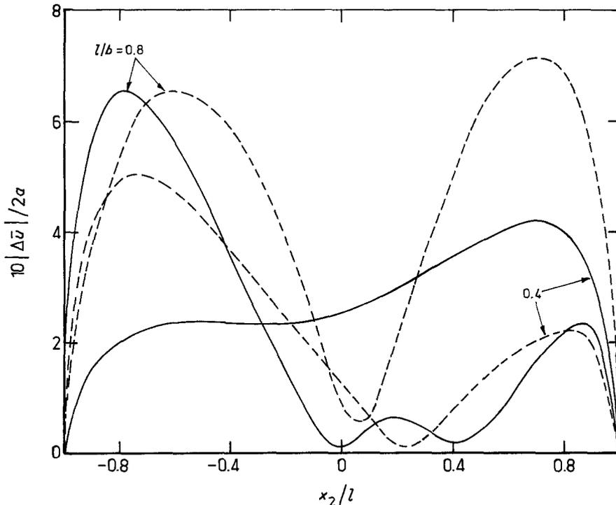
Figure 9 Relative displacements across the debonded faces corresponding to the strain (Equation 62).  $\lambda_1/\lambda = 20$ ,  $b/a = 0.8$ ,  $\nu = \nu_1 = 0.3$ . Normal displacements are shown by solid lines and tangential displacements by broken lines.
