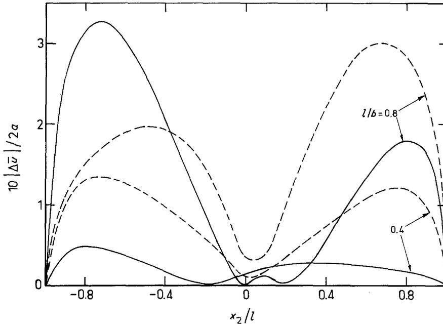
Figure 8 Relative displacements across the debonded faces corresponding to the strain (Equation 62).  $\lambda_1/\lambda = 20$ ,  $b/a = 0.4$ ,  $\nu = \nu_1 = 0.3$ . Normal displacements are shown by solid lines and tangential displacements by broken lines.
