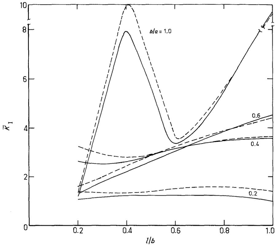
Figure 2 Stress-intensity factor  $\bar{K}_I$  corresponding to the applied strain (Equation 60).  $\lambda_1/\lambda = 20$  (solid lines) and  $\lambda_1/\lambda = 50$  (broken lines). In all cases,  $\nu = \nu_1 = 0.3$ .
