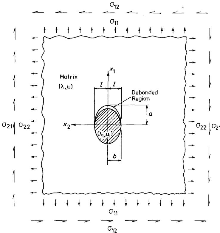
Figure 1 The debonded elliptic inhomogeneity, showing the coordinate axes and the remote stress-field.
