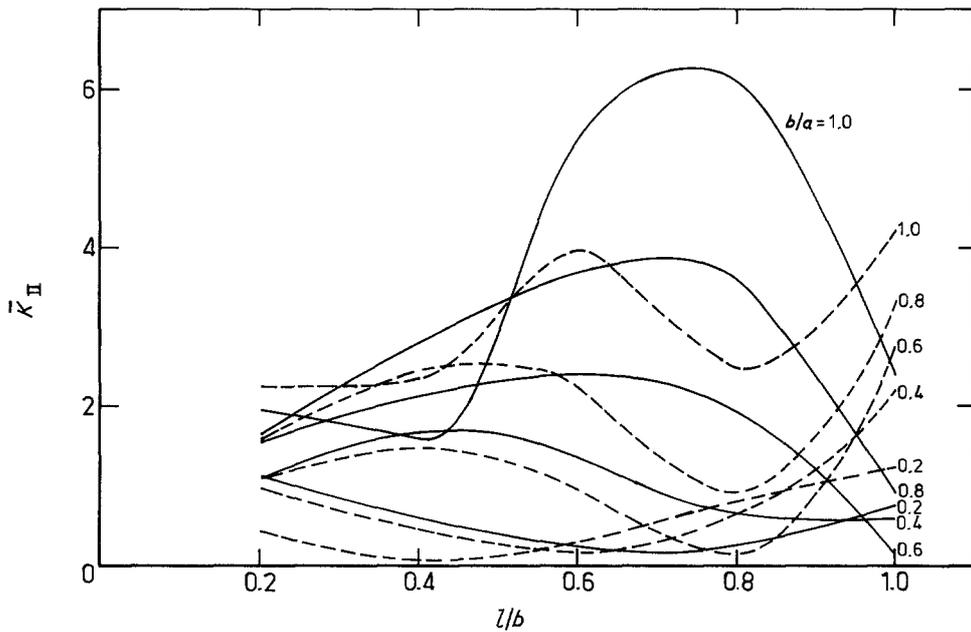
Figure 7 The stress-intensity factor  $\bar{K}_{II}$  for the applied strain (Equation 62).  $\lambda_1/\lambda = 20$ , and  $\nu = \nu_1 = 0.3$ . (Solid lines represent  $x_2 > 0$  side of the debond and broken lines  $x_2 < 0$  side of the debond.)
